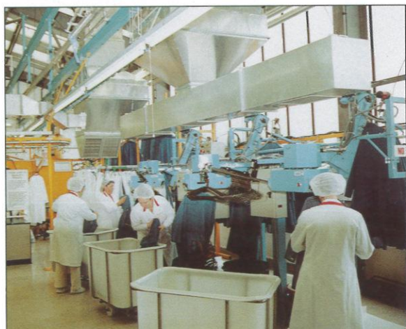
FENLAND LAUNDRIES, GRANTHAM - Local air inlet with hepa filters to clean room.
